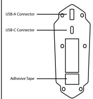
NOTE: Peel the adhesive tape on the bottom of the USB hub extender so it adheres to the PS5 better. This will ensure that it will stay securely on your PS5.
