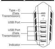
NOTE: The regular USB port (non-data transmission port) can only charge. It does not support data so it can only be used as a USB port to charge your devices. The other USB ports (data transmission supported ports) support data transmission, so they can be used to charge and also for data transfers.
